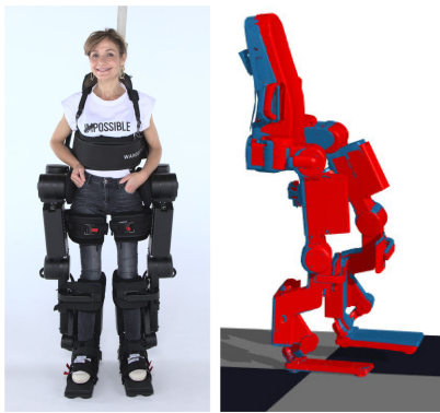
Fig. 1. Picture of the exoskeleton Atalante with a paraplegic user. On the right, CAD reconstruction under the assumption of full rigidity (blue), and ground truth from motion capture (red): the real robot is leaning forward due to deformations.
