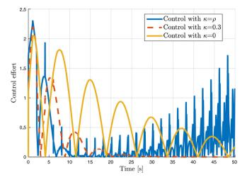
**Fig. 5.** Time evolution of the control effort U(t) for different values of  $\kappa$  in presence of a 0.02 s delay.
