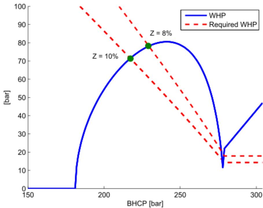
Figure 5: Operating envelope showing operating points for the choke openings: Z=10% and Z=8%.
