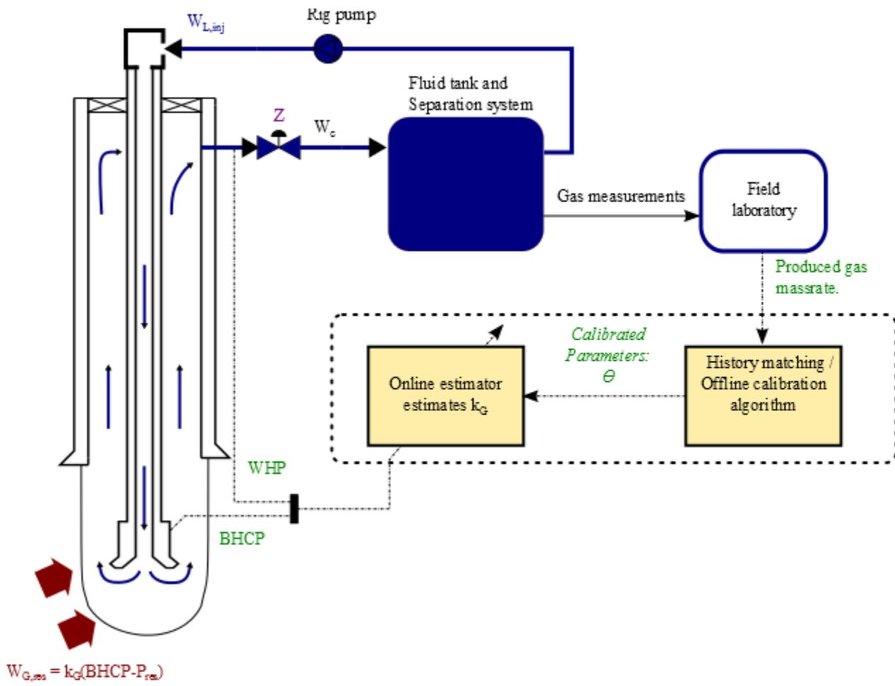
Figure 1: Process schematic of the proposed architecture.
