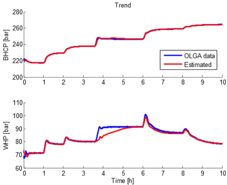
Figure 3: Measured WHP and BHCP used to estimate PI.
