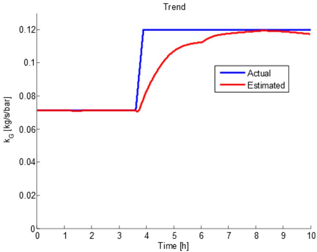
Figure 2: Estimating PI using only pressure measurements.
