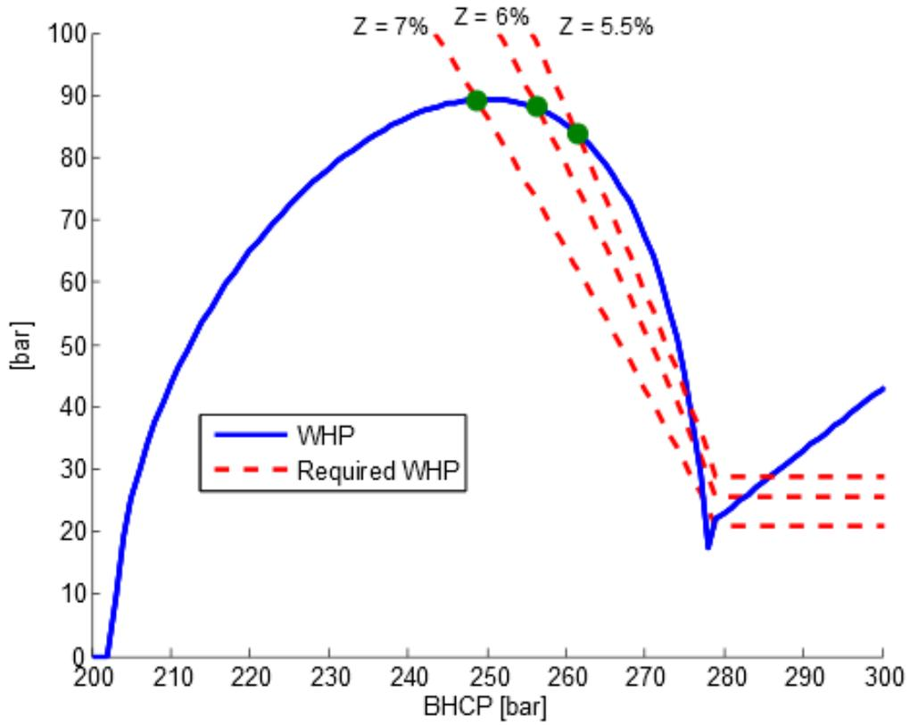
Figure 6: Updated operating envelope after the increase in the production index.
