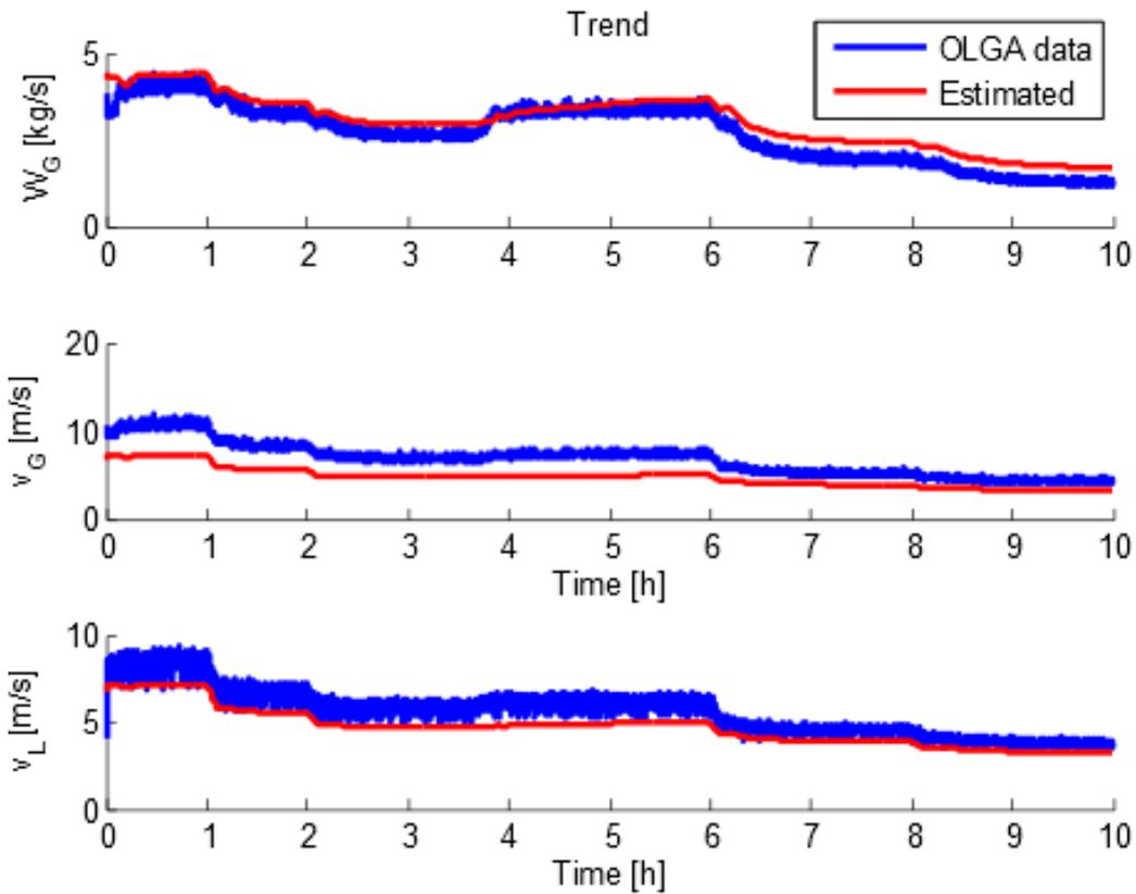
Figure 4: Unmeasured OLGA data and estimated gas mass rate and gas and liquid velocities at the wellhead.
