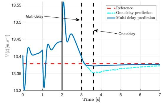
Fig. 4. Axial velocity of the BHA. The solid black line corresponds to the time instant when the controller is switched on. The dashed black line corresponds to the time instant when the control kicks in.
