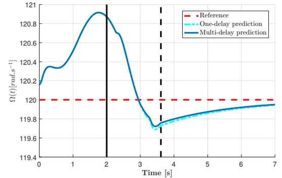
Fig. 5. Torsional velocity of the BHA. The solid black line corresponds to the time instant when the controller is switched on. The dashed black line corresponds to the time instant when the control kicks in.
