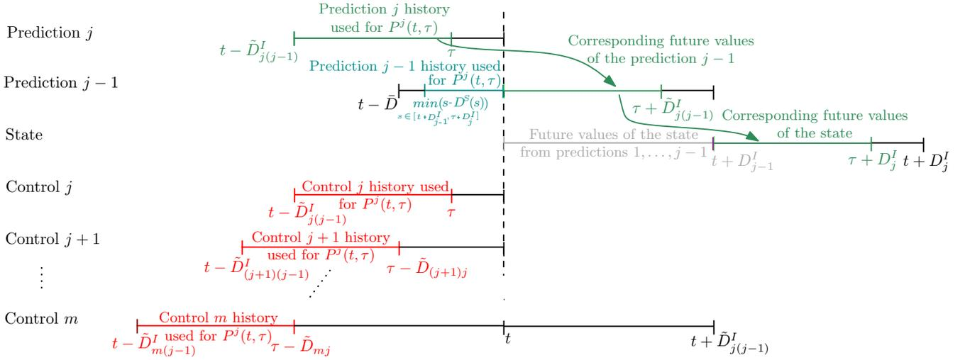
Fig. 2. Schematic view of the variables involved in the computation of the prediction  $P^j(t, \tau)$ . Consequently, the computation of  $P^m(t, \tau)$  involves the history of  $X$  over  $[\min_{s \in [t, \tau + D_m^I]}(s - D_m^I), t]$  (which is included in  $[t - \bar{D}, t]$ ), of  $U_j$  over  $[t - D_j^I, t]$  for  $j = 1, \dots, m-1$  and of  $U_m$  over  $[t - D_m^I, \tau]$ .
