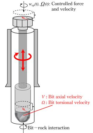
Fig. 3. Schematic view of drilling facilities.
