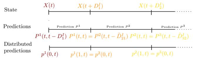
Fig. 1. Schematic view of the predictions defined in (16)–(17) and corresponding future values of the state. Distributed predictions involved in the proof of Theorem 1 and defined in (36), (39) are also depicted.
